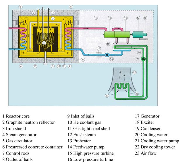
The refuelling machine built into the reactor vessel made it possible to replace the spent fuel balls with new ones during operation. In THTR-300 approximately 620 balls were replaced by fresh ones every day; the balls spent 3 years in the reactor and during this period they passed through the core six times.
