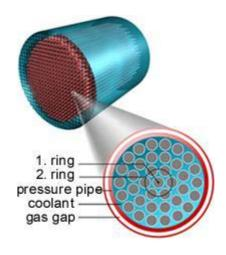
The other type of heavy water reactor is the pressurized heavy water reactor (PHWR). In this type the moderator and coolant are the same and the reactor pressure vessel has to stand the high pressure.
